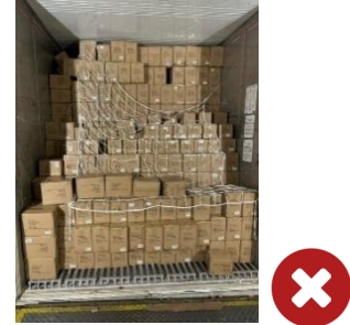
Example of how not to pack a container
